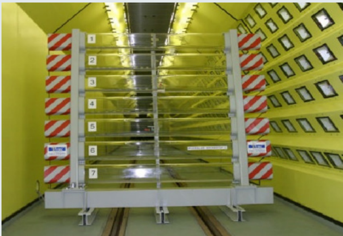
ACRYLITE® Soundstop Wind Barrier panels undergoing a wind tunnel test for efficacy & wind deflection
