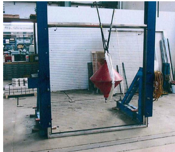
ACRYLITE® Soundstop GS CC with framing system for EN 1794-2, Annex B test
