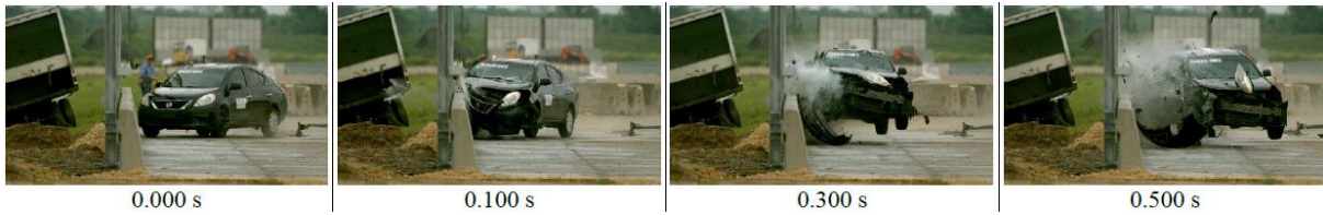
Time-lapse of MASH 4-10 (TL-2) crash test
