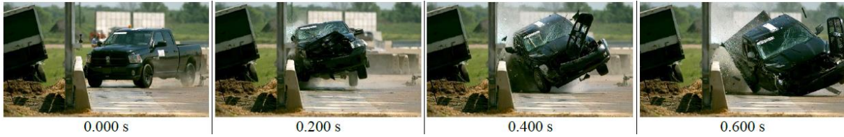
Time-lapse of MASH 4-11 (TL-3) crash test
