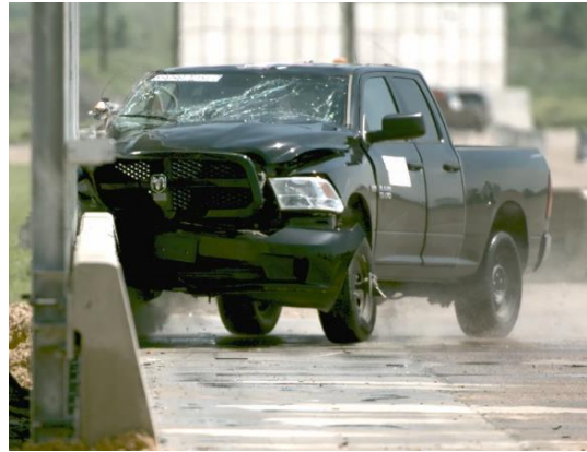
Still image of the heavy duty pick-up truck used in the TL-3 MASH Crash Test at Texas A&M Transportation Institute Proving Ground, College Station, TX.
