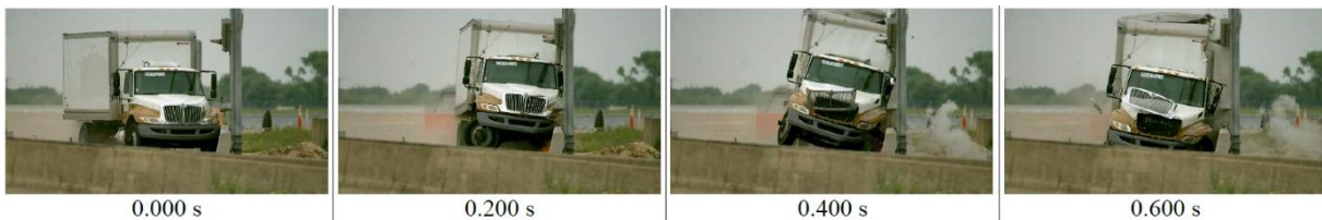
Time-lapse of MASH 4-12 (TL-4) crash test
