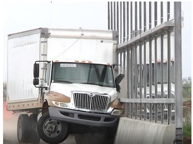
MASH Test 4-12 uses a 22,180 lb box truck at 58 mph at a 15° angle which meets the minimum TL-4 criteria of 142 kip-ft.
