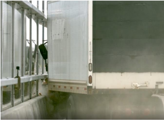
Still image of the box truck used in the TL-4 MASH Crash Test at Texas A&M Transportation Institute Proving Ground, College Station, TX.
