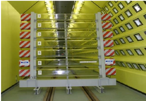
ACRYLITE® Soundstop Wind Barrier panels undergoing a wind tunnel test for efficacy & wind deflection
